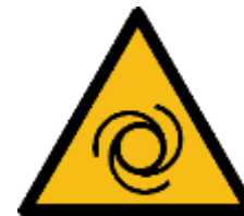
Remotely Started Equipment
