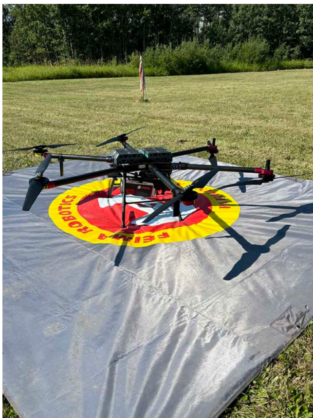
A FEMIA Robotics D20 Drone with Riegl Lidar Sensor VUX-120 during a site search in 2024 (Office of the Independent Special Interlocutor).
