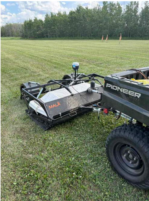
A Mala Mira HDR Multi-Chanel Ground Penetrating Radar machine being towed across search area (left), and an S4 Subterra Gray Soil Spectroscopy machine (right) during a ground search in 2024 (Office of the Independent Special Interlocutor).
